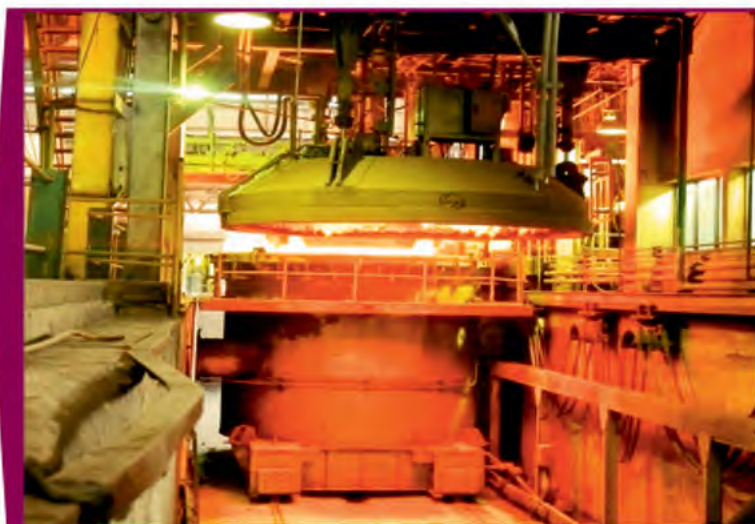
20 MT LADLE FURNACE & VACUUM DEGASING - USED FOR SECONDARY REFINING
